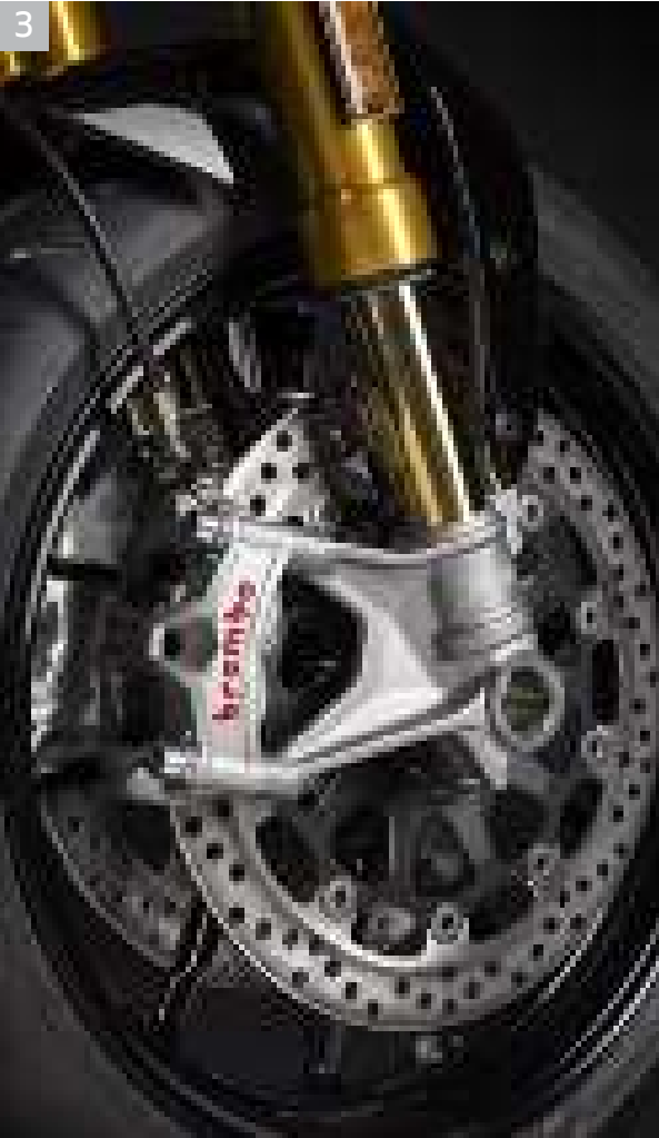
3 Radially mounted Brembo Stylema® monobloc 4-piston callipers
